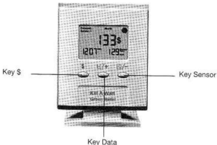
Three operational buttons are provided on the device. They are allocated with two functions selected with a short/long press of the button. The two buttons on the right can also be used as value input buttons depending on the context.
