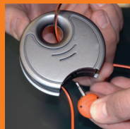
Remove the key for activation (insert again for deactivation or turn off the alarm)
