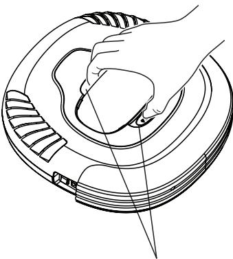
Grip slot for the dust bin
